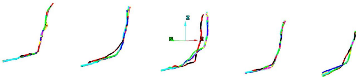
Figure 10 – Cross-sections, at 50 m spacing, for South section: Red = 2010, Black = 2012, Blue = 2017, Green = 2019, Yellow = 2020, Fuchsia = 2021, Cyan = 2022 (Extents: E 567329 m, N 341540 m to E 567272 m, N 341359 m)
