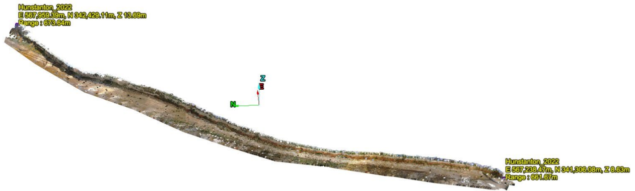
Figure 4 – 2022 point cloud data displayed using the RGB colour values (Extents: E 567959 m, N 342429 m to E 567238 m, N 341306 m. Height range = 6.3 m to 18.8 m)
