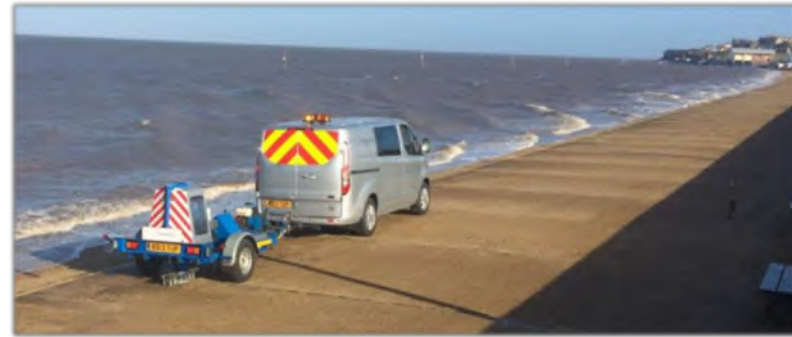
Falling weight deflectometer survey being undertaken in 2015
