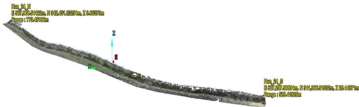
Figure 4 – 2024 point cloud data displayed using the RGB colour values (Extents: E 567969 m, N 342451 m to E 567288 m, N 341366 m. Height range = 6.3 m to 18.8 m)
